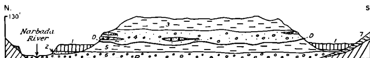
FIGURE 182.—Composite transverse section through Narbada Valley near Narsinghpur. 1, cotton soil; 2, basal gravel of cotton soil; 3, 4, upper group with pink concretionary clay (3) and upper gravel and sand (4); 5, 6, lower group with red concretionary clay (5) and basal conglomerate (6); 7, laterite; D, disconformity between upper and lower groups.
